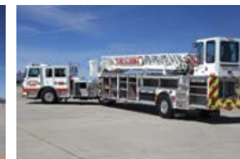
60° jack-knife angle & 500 cubic feet of compartment storage
